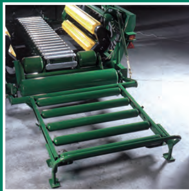
998 Unloading Conveyor Down
