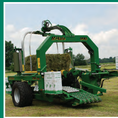
Lifting Bale to Wrapping Position
