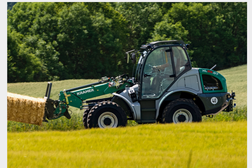
Front wheel steering for increased stability during quick transport trips
