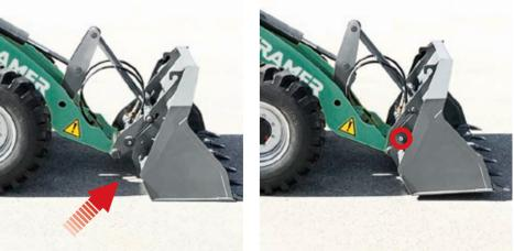
the operator's seat and lock it using the touch slide on the joystick. The lock cylinder is located above of the pivot point of the quickhitch plate and is thus not in the contamination area.
