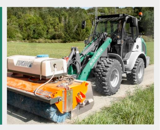
**CSD** - constant travel speed: supports compliance with the set speed, especially when running attachments where a consistent speed is required for the correct execution of the work process, such as: snowblower protection, rotary sweeper or mulcher.
