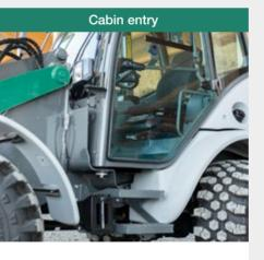
The cabin can be accessed through the large entry area. A two-stage entry is optionally available to give the operator an even more comfortable entry.\* In addition, the handles are in an ergonomically favourable position.
