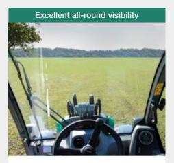
The central seat position in combination with the large glass windows offer a 360° all-round visibility. The particularly clearlyarranged design and the seat position of the operator avoid "blind spots". You can even see everything to the rear. The elevated front window allows for a perfect view of the attachment, even when the loader unit is raised.
