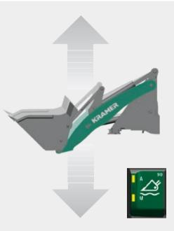
The load stabiliser dampens oscillations of the load stabilizer, providing for improved ride comfort and increased driving safety.
