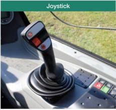
The ergonomically shaped joystick is securely integrated into the armrest and allows for sensitive and precise machine control. The speed selection is right on the joystick to increase the level of convenience. This makes it possible to switch over between the two speeds faster.
