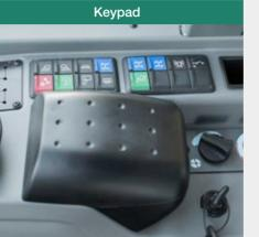
The respective functional group is very quick and easy to identify due to the colour-coded switches. Red = safety, green = hydraulics, blue = travel and grey = electrical system. This ensures the operator a convenient and safe operation without the risk of being confused. The result is increased working efficiency.
