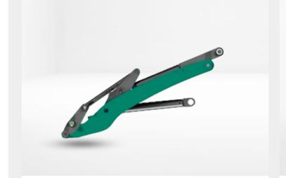
The parallel-guided loader unit ensures constant lift capacity and a safe operation in materials handling. Due to the 50° high tilt back angle and the tilt-out angle of 45°, the wheel loader does not lose any material in bucket application, even when it is very full, allowing for a complete emptying of the bucket.
