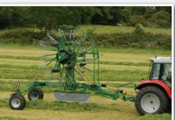
For transport, when the rotors are folded up, they move down into a locking position, which delivers a transport height under 4 meters. As a result, tine arms do not need to be removed for transport. The McHale R 62-72 & R 68-78 are equipped as standard with 380/55 -17 wide tyres, which give excellent stability on the road, while minimising compaction in the field. The transport running gear is approved up to 40 km/ h.
