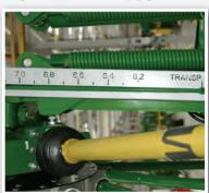
The McHale R 62-72 & R 68-78 twinrotor centre delivery rakes offer a number of different working widths as illustrated in the table above. The variable working width is adjusted hydraulically from the tractor seat.
