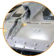
**Hydraulically controlled rear door**
